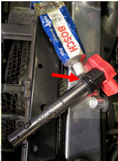
Figure 1 - Lubricate the lip of the ignition coils
