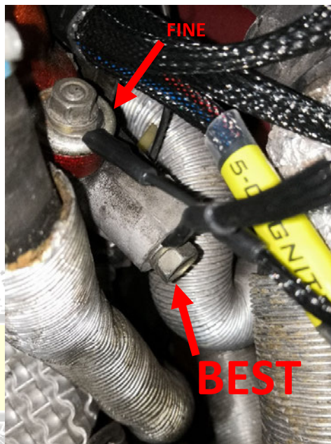
Figure 5 – Ground wire bolt down points
