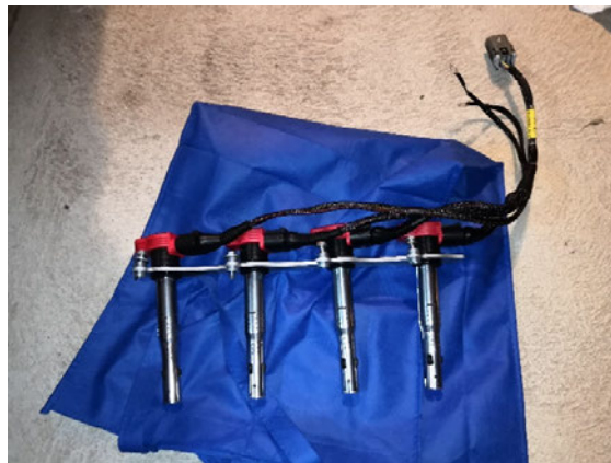
Figure 2- Pre-assembling coils and harness into the mounting plate
