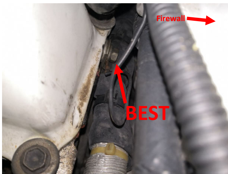
Figure 6 – Bolt down the other ground wire ring on stock ground position behind the head
